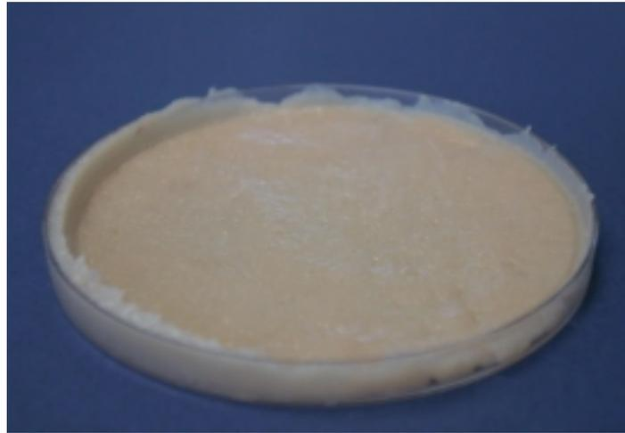
Spoilt sample after 10 d at  $4\pm 1^\circ\text{C}$
