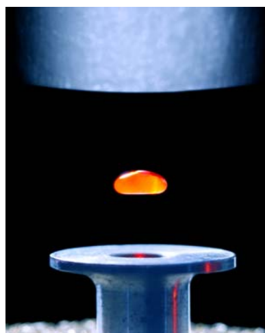
Fig 1. 5 \mu L acoustic levitated drop of erythrocytes irradiated with 780 nm laser
