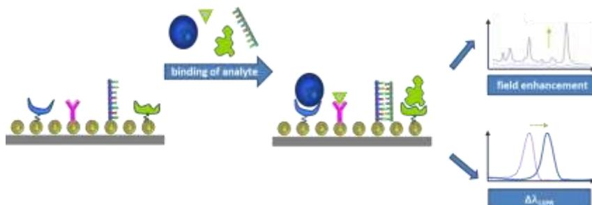
Figure 1: Nanoparticles with recognition element serve as LSPR and SERS sensor respectively. Binding of analyte to recognition elements attracts attention to spectral shift and field enhancement respectively.
